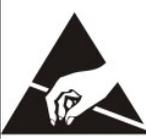
**Electrostatic discharge can affect electronic components. Take precautions to neutralize electrostatic charge by touching your hand and tools to metal prior to handling the control.**
