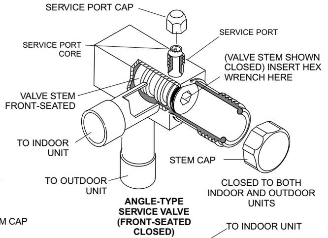
WHEN SERVICE VALVE IS CLOSED, THE SERVICE PORT IS OPEN TO THE LINE SET AND INDOOR UNIT.
