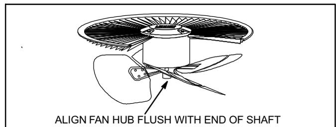
**Figure 2. Fan Hub Alignment.**
