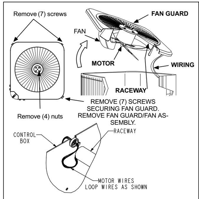
**Figure 1. Condenser Fan Motor and Compressor Access**
