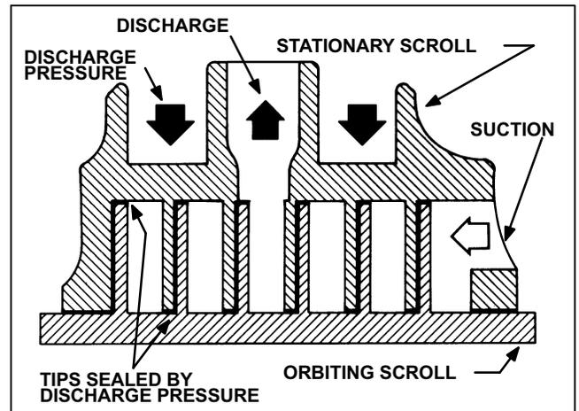
Figure 5. Scroll Cross-Section
