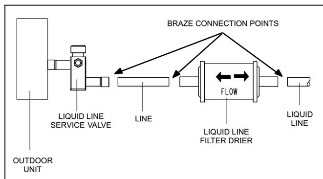
**Figure 10. Typical Bi-Flow Liquid Line Filter Drier Installation**
