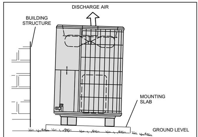
Figure 9. Typical Slab Mounting at Ground Level
