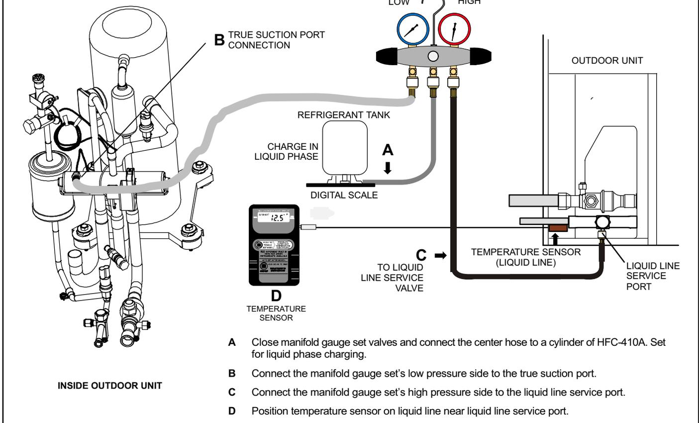
**Figure 13. Gauge Set Setup and Connections**
