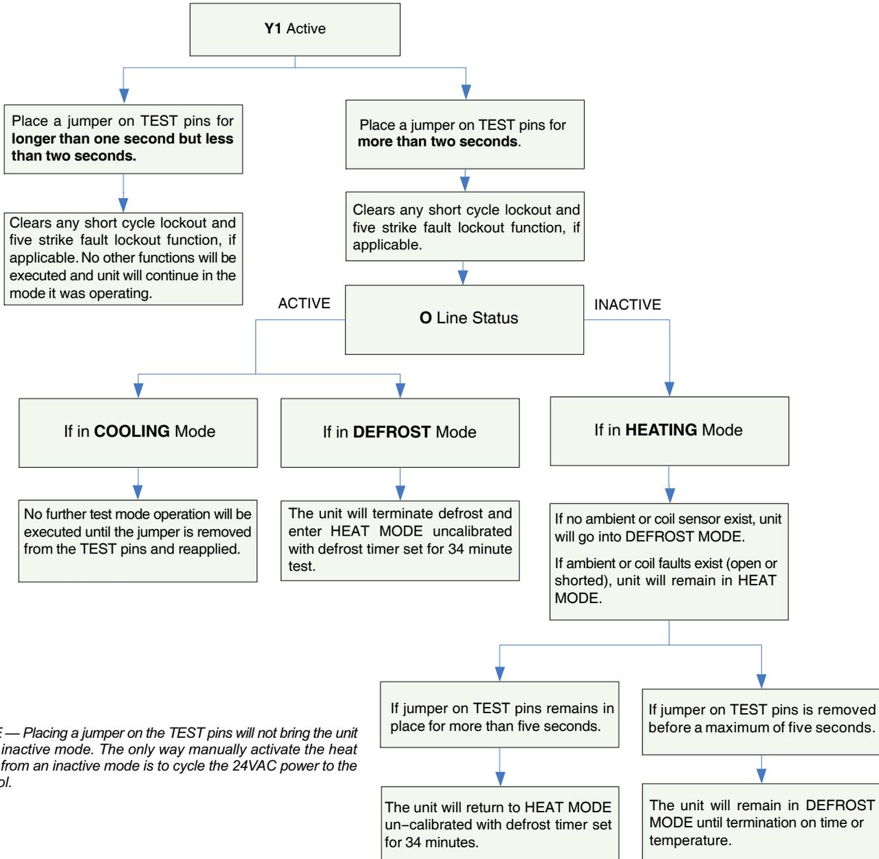
*NOTE — Placing a jumper on the TEST pins will not bring the unit out of inactive mode. The only way manually activate the heat pump from an inactive mode is to cycle the 24VAC power to the Control.*
