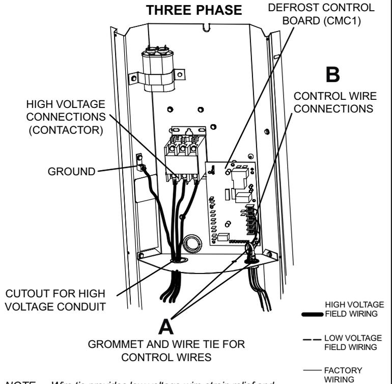
*NOTE* — Wire tie provides low voltage wire strain relief and to maintain separation of field installed low and high voltage circuits.
