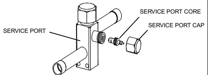
**WARNING** — Allow braze joint to cool before removing the wet rag from the service valve. (TEMPERATURES ABOVE 250°F CAN DAMAGE VALVE SEALS)
