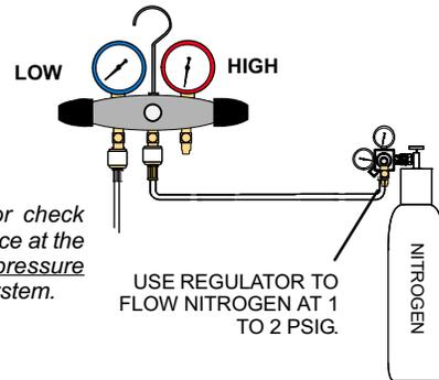
**NOTE** — The fixed orifice or check expansion valve metering device at the indoor unit will allow low pressure nitrogen to flow through the system.
