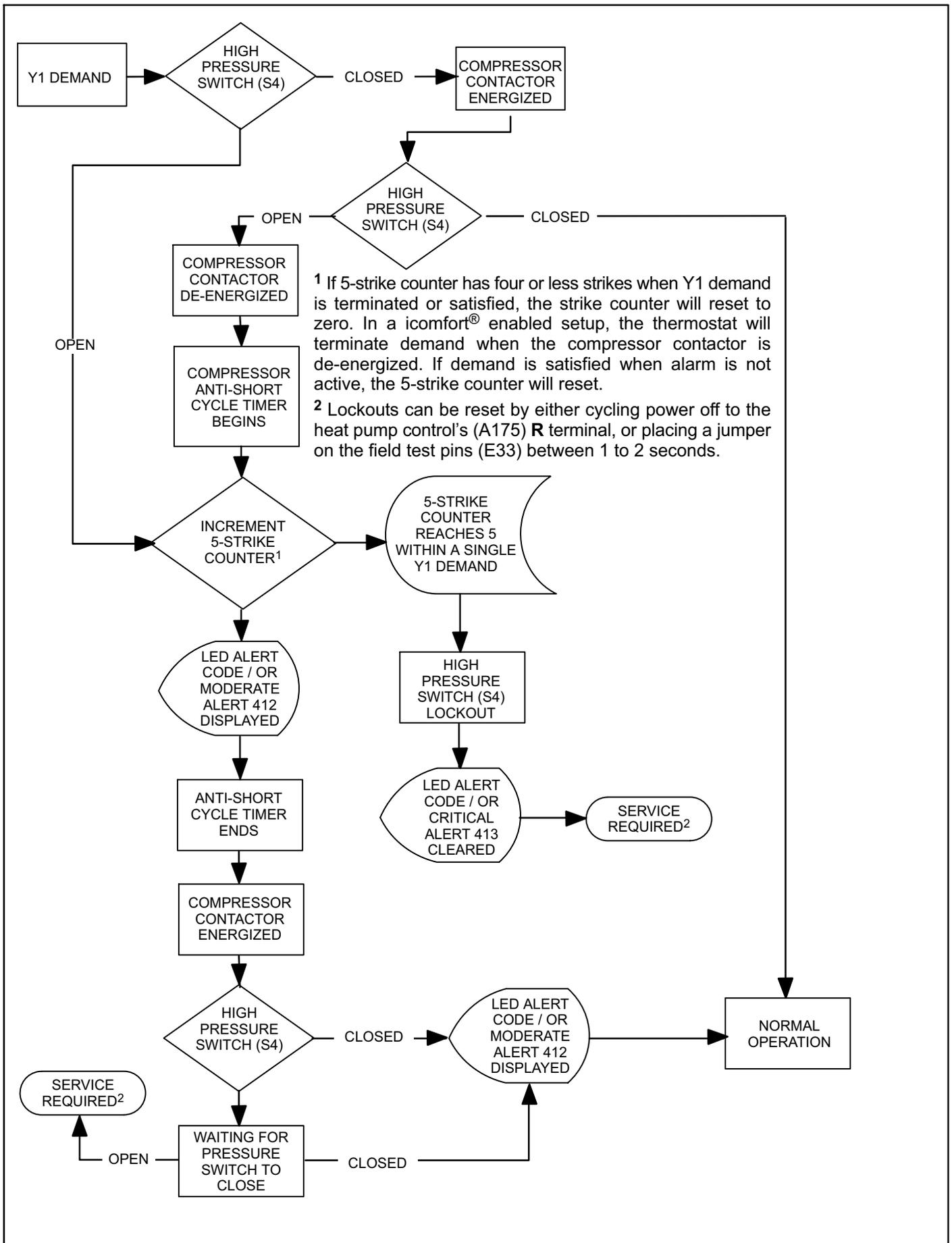
Figure 33. High Pressure Switch (S4) Sequence of Operation
