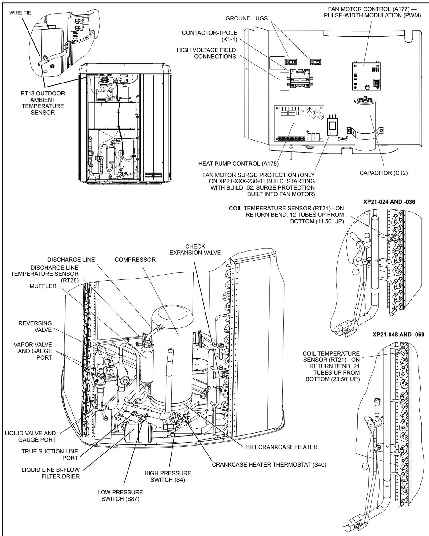
Figure 1. Plumbing, Switches and Sensor Components
