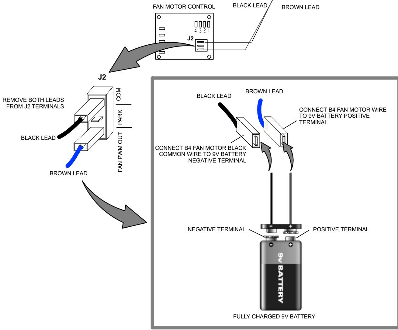
Figure 24. B4 Fan Motor Test
