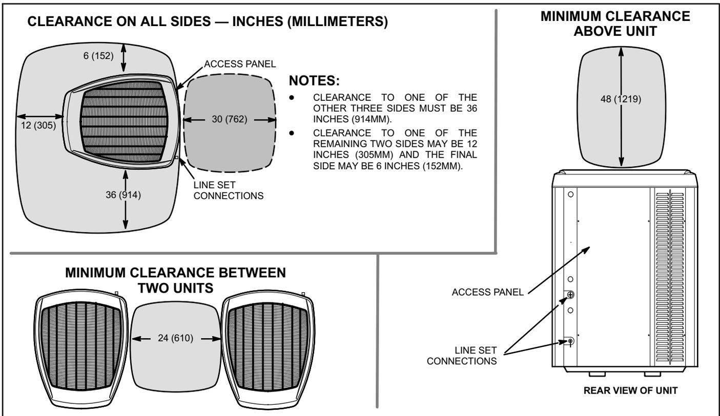
Figure 3. Installation Clearances
