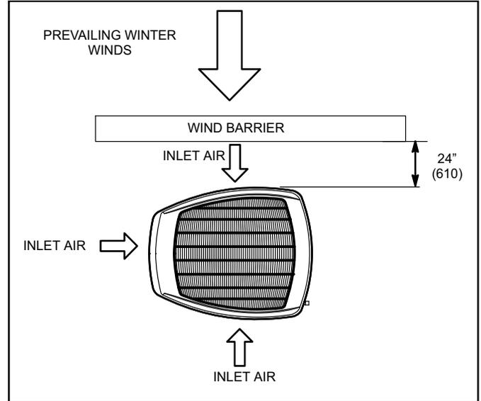
Figure 4. Rooftop Application and Wind Barrier
