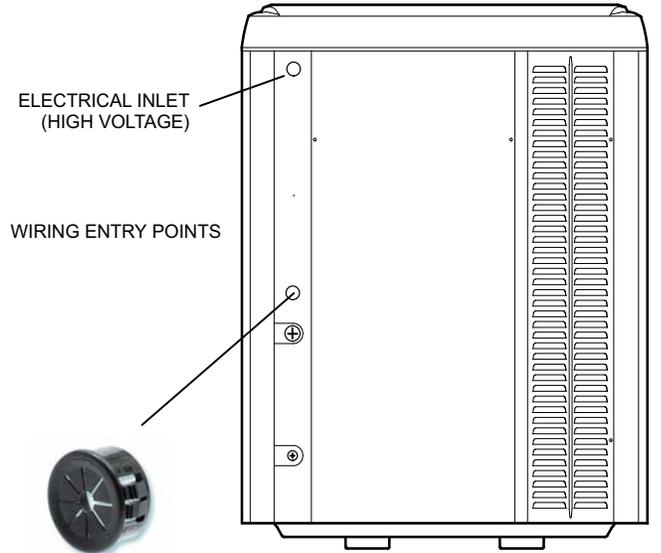
ELECTRICAL INLET (CONTROL WIRING — LOW VOLTAGE). USE BUSHING PROVIDED IN BAG ASSEMBLY HERE.
