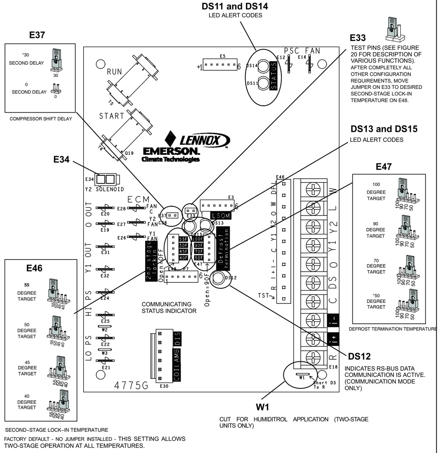
Figure 13. Heat Pump Control Connections, Jumper Settings and LED Locations
