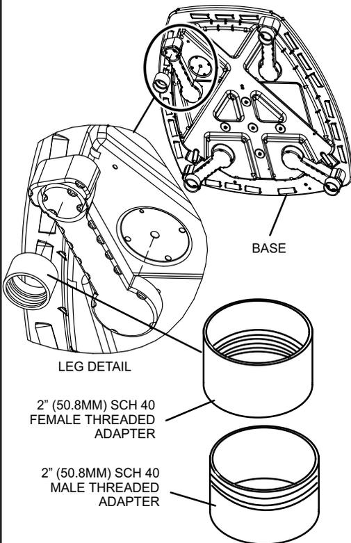
USE ADDITIONAL 2" SCH 40 MALE THREADED ADAPTERS WHICH CAN BE THREADED INTO THE FEMALE THREADED ADAPTERS TO MAKE ADDITIONAL ADJUSTMENTS TO THE LEVEL OF THE UNIT.
