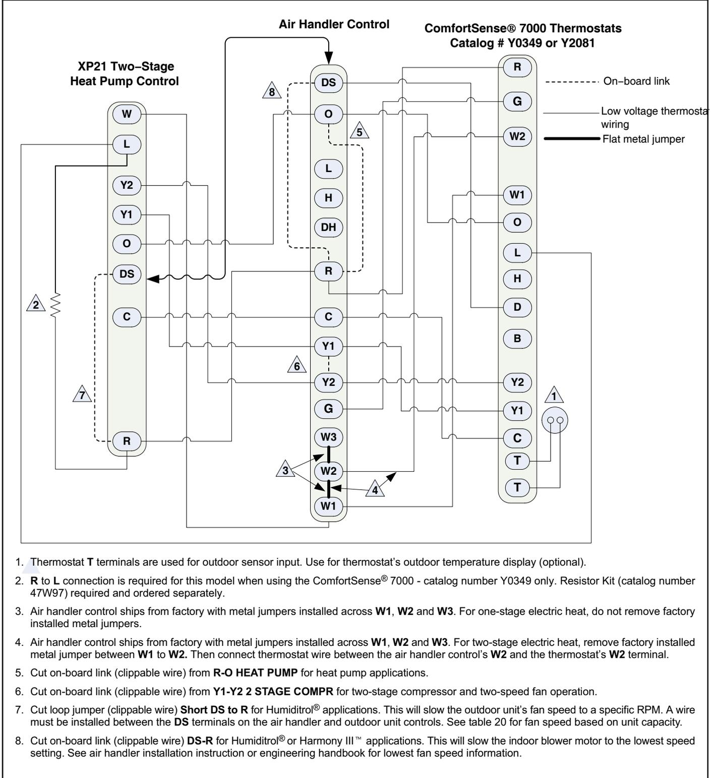
**Figure 14. ComfortSense® 7000 Series Thermostat — Air Handler/Two-Stage Heat Pump**
