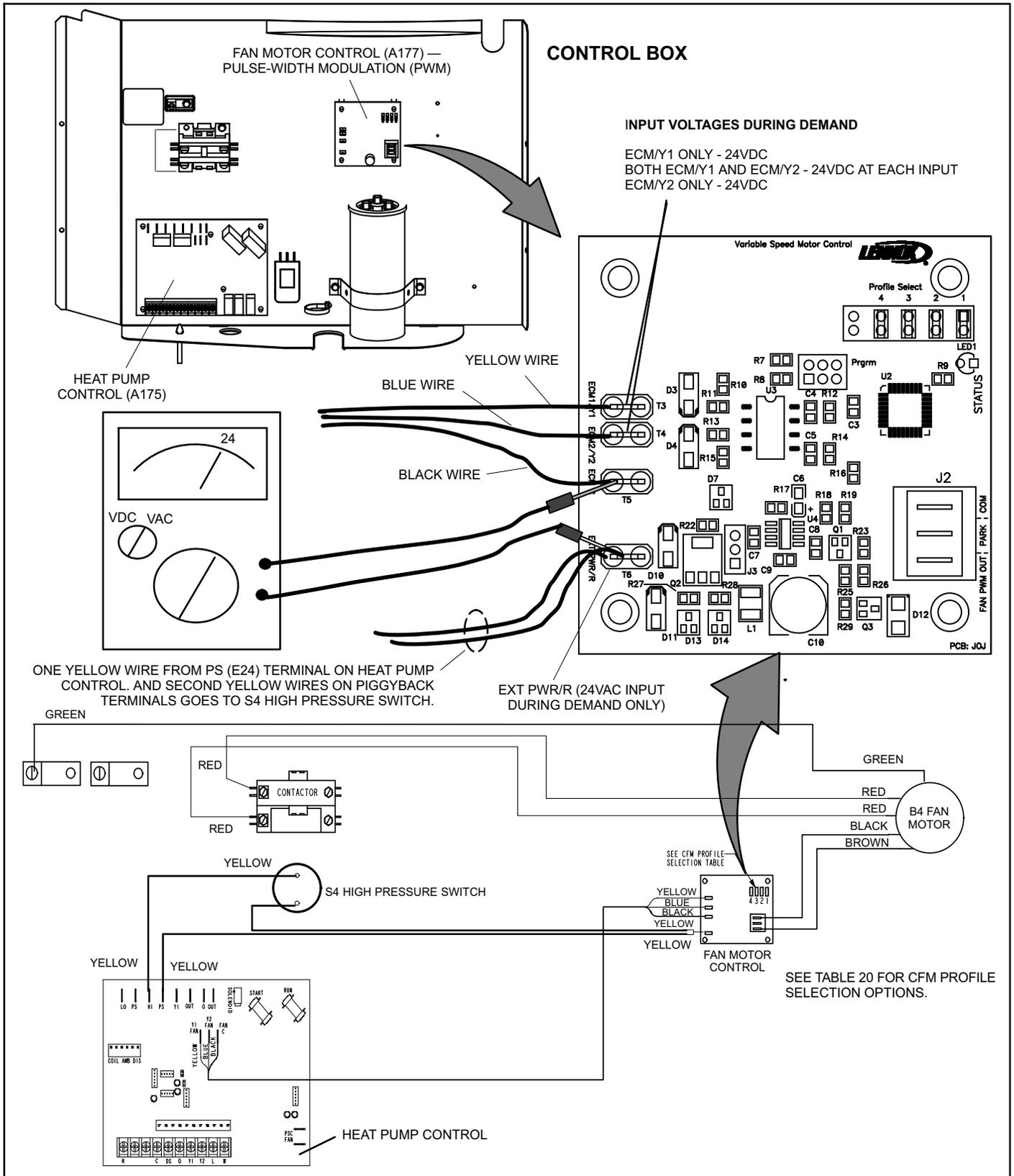
Figure 23. Testing for External Power to Fan Motor Control (A177)
