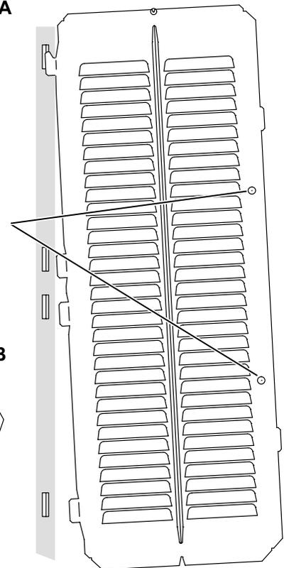
ROTATE IN THIS DIRECTION; THEN DOWN TO REMOVE PANEL
