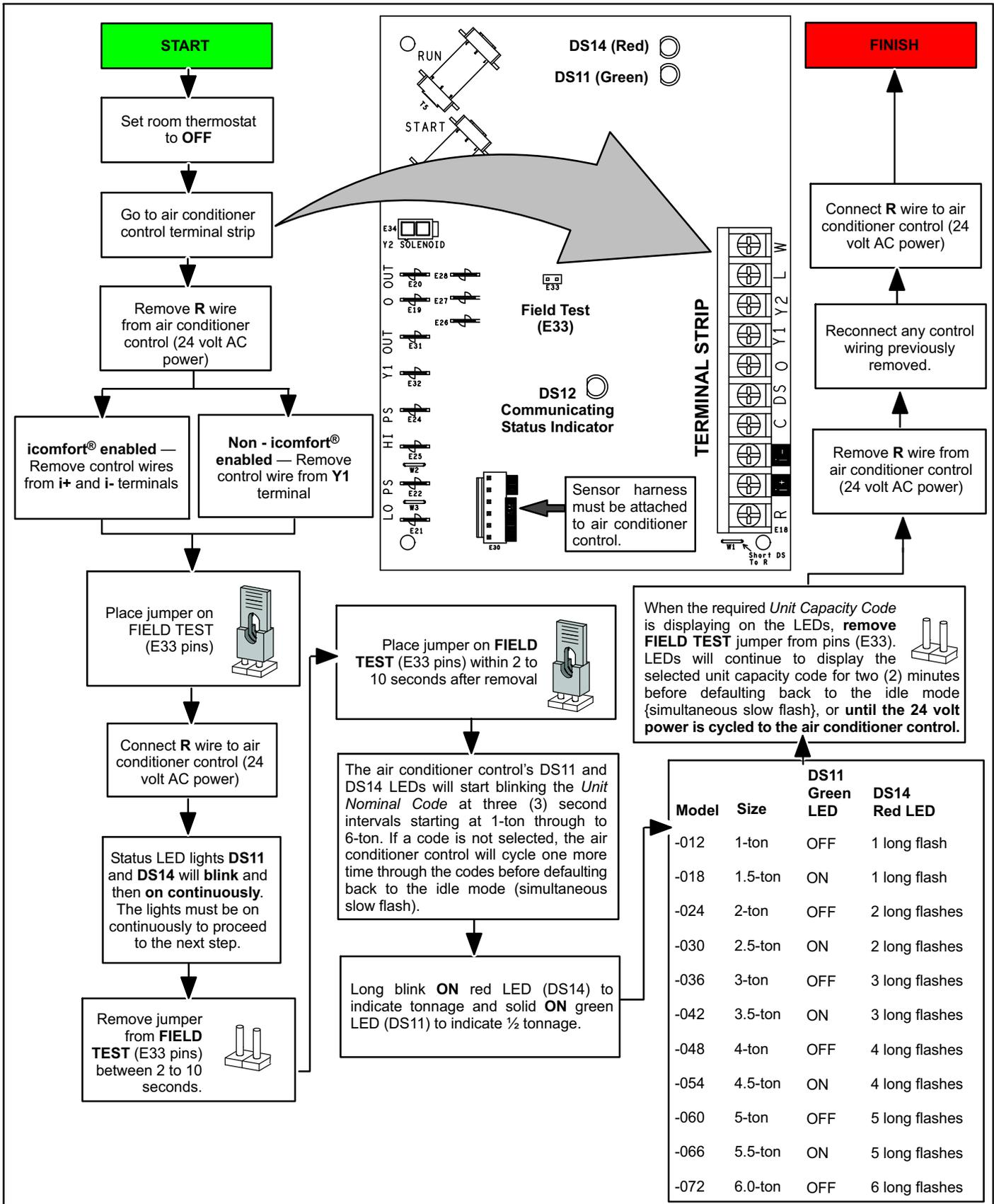
Figure 26. Heat Pump Control (A175) Unit Nominal Capacity Code Configuration
