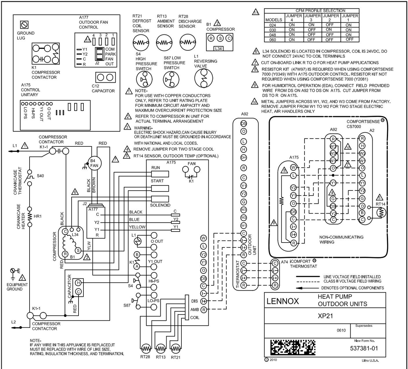
Figure 30. Typical XP21 Wiring (XP21-XXX-230-02 only)
