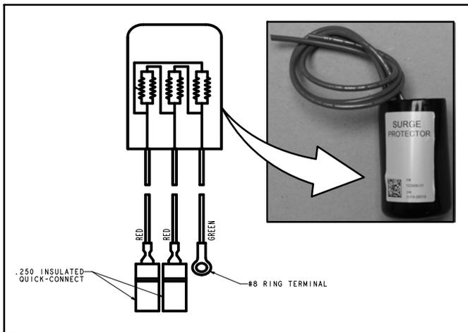
**Figure 27. Fan Motor Surge Protection Device
