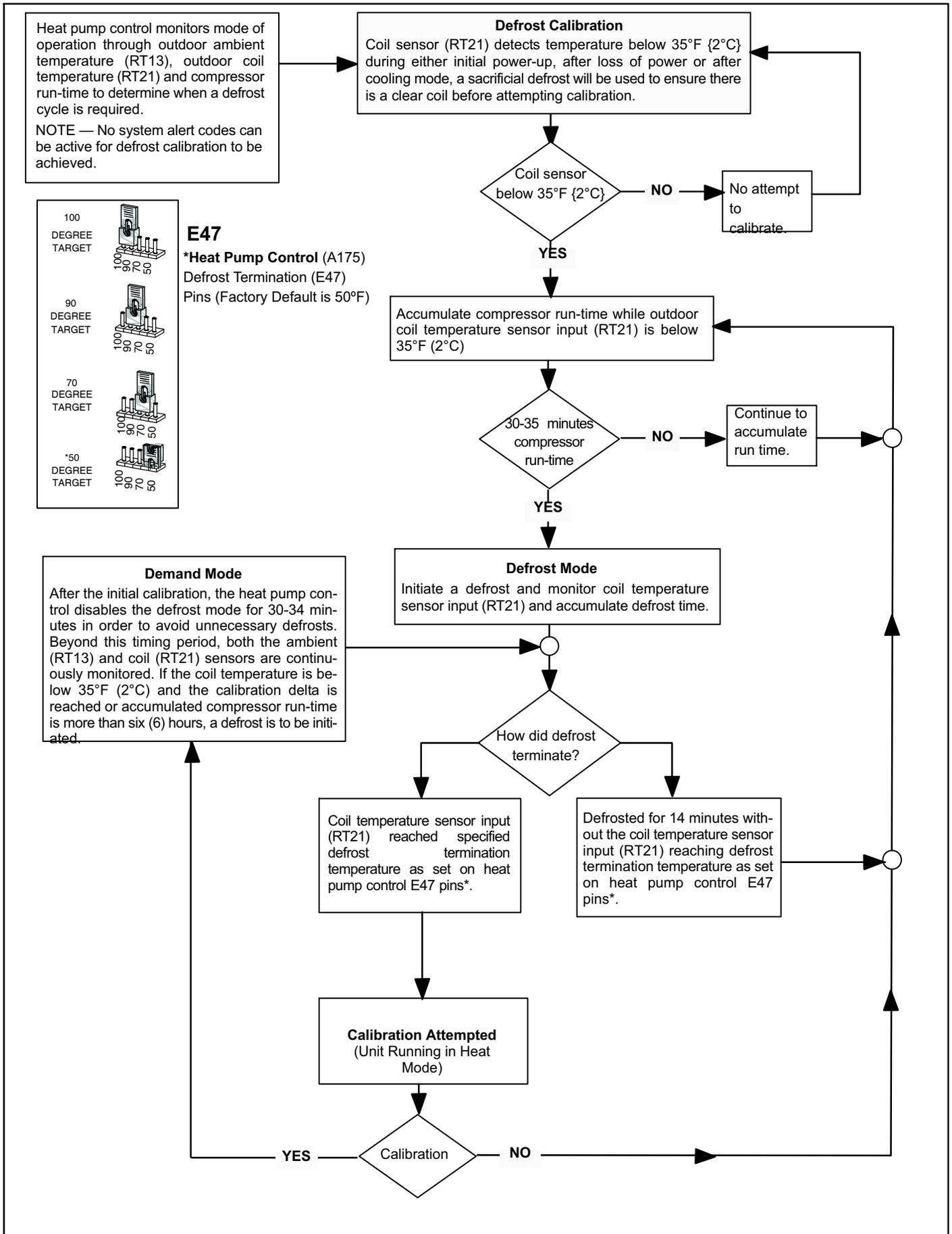
Figure 35. Defrost Calibration and Defrost Mode Sequence of Operations
