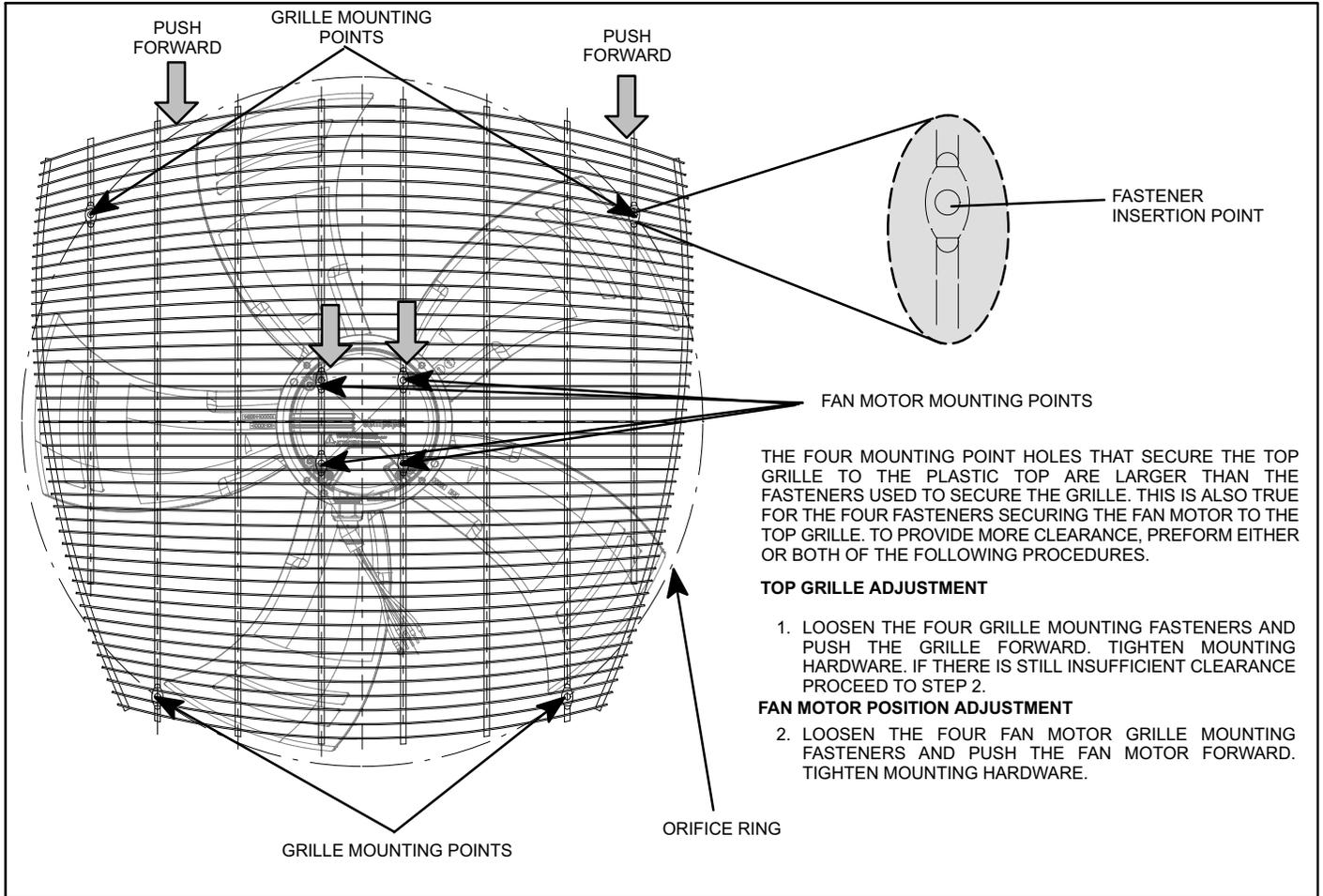
Figure 25. Fan Blade Clearance Adjustment
