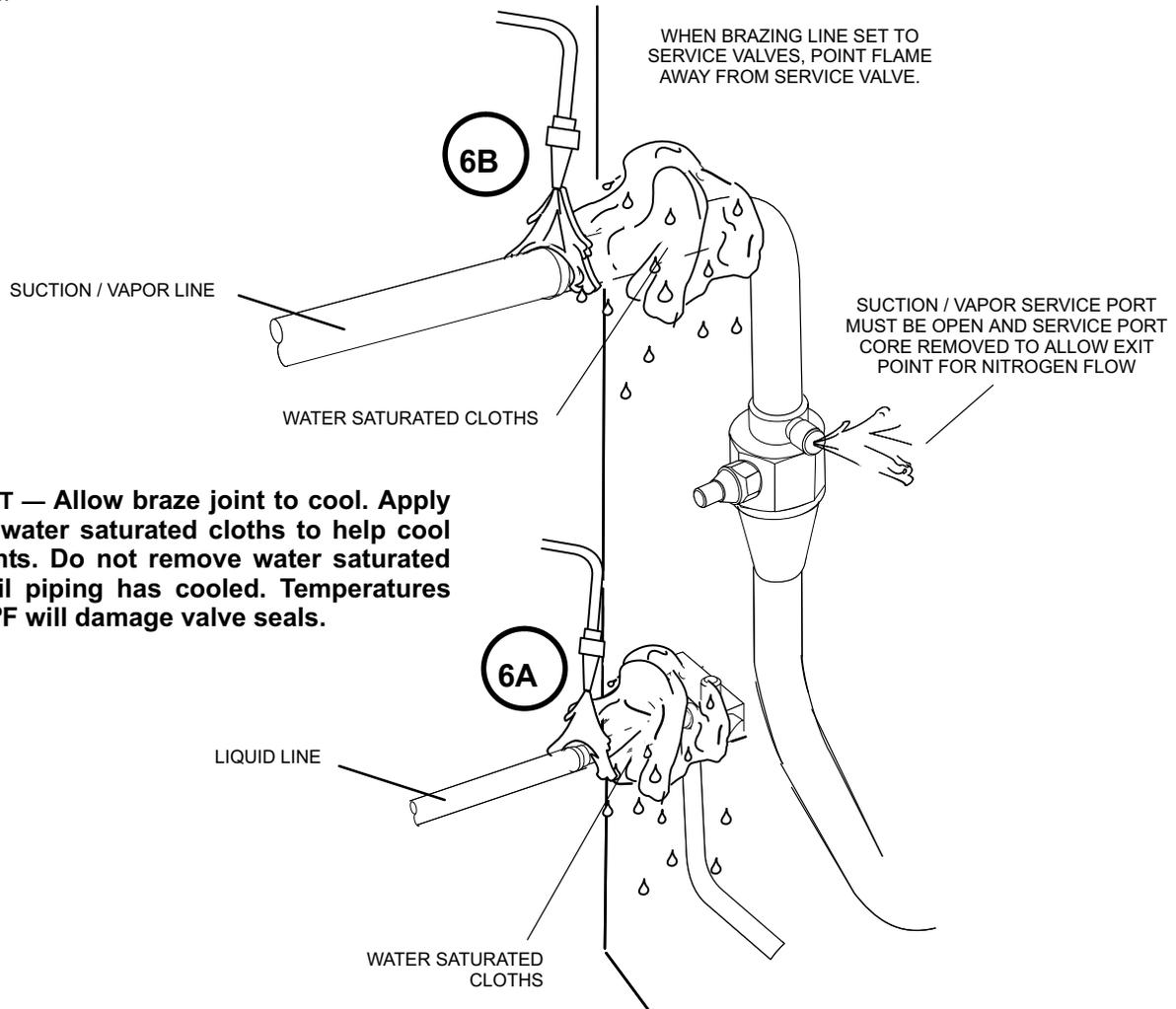
**IMPORTANT — Allow braze joint to cool. Apply additional water saturated cloths to help cool brazed joints. Do not remove water saturated cloths until piping has cooled. Temperatures above 250°F will damage valve seals.**
