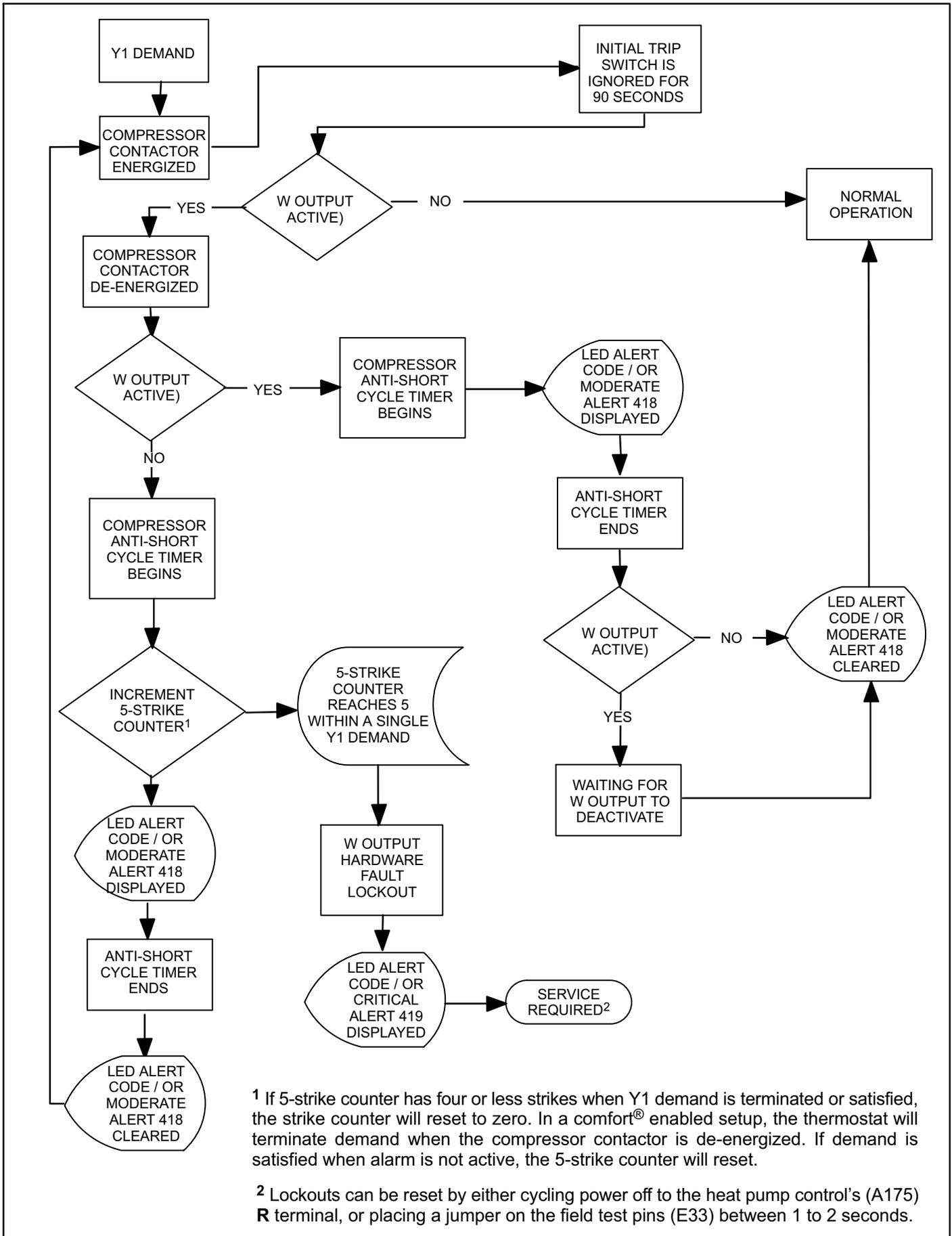
**Figure 36. W Input Fault or Miswire Sequence of Operation**
