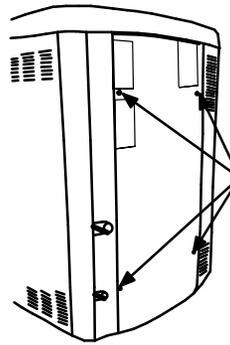
REMOVE 4 SCREWS TO REMOVE PANEL FOR ACCESSING COMPRESSOR AND CONTROLS.
