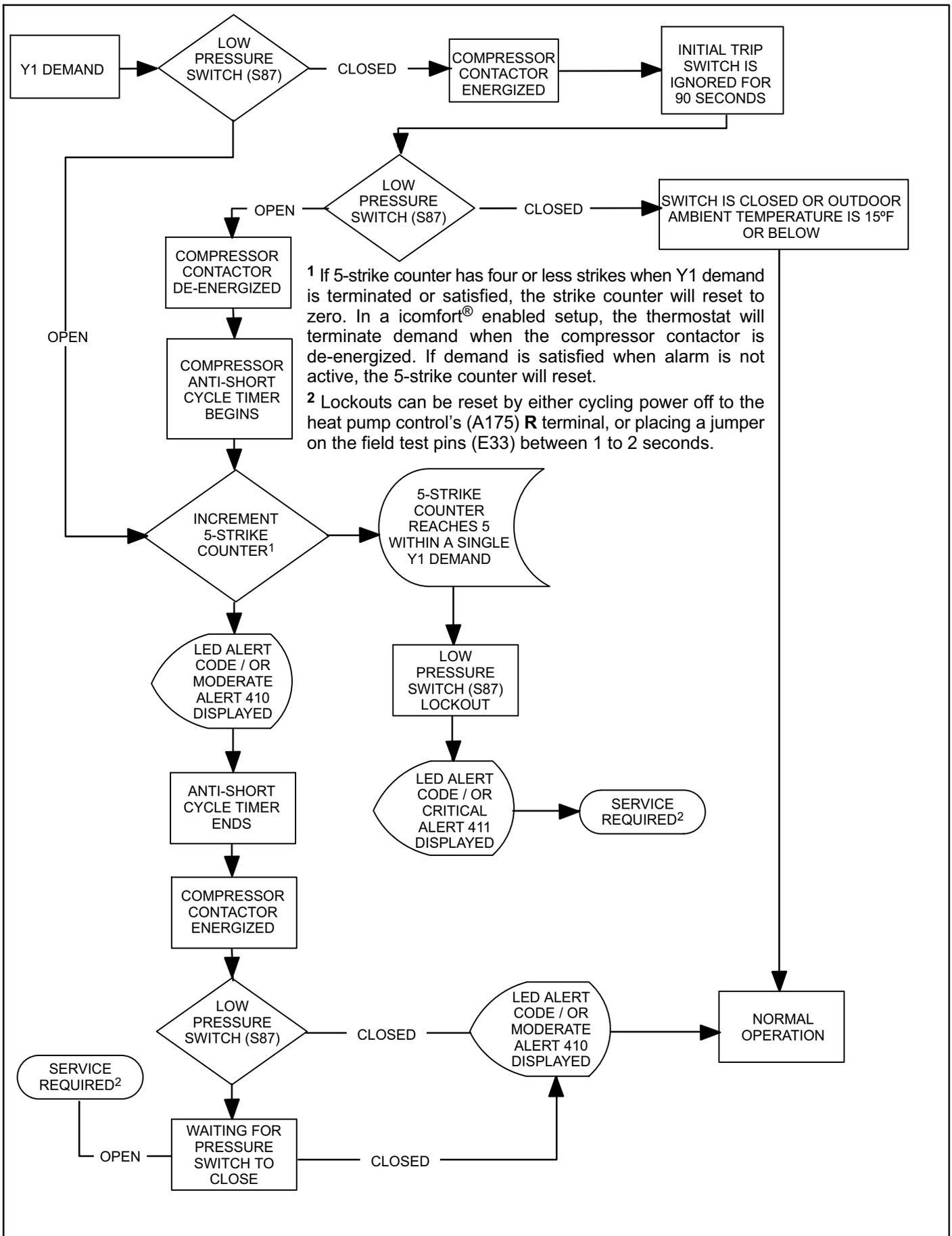
Figure 32. Low Pressure Switch (S87) Sequence of Operation
