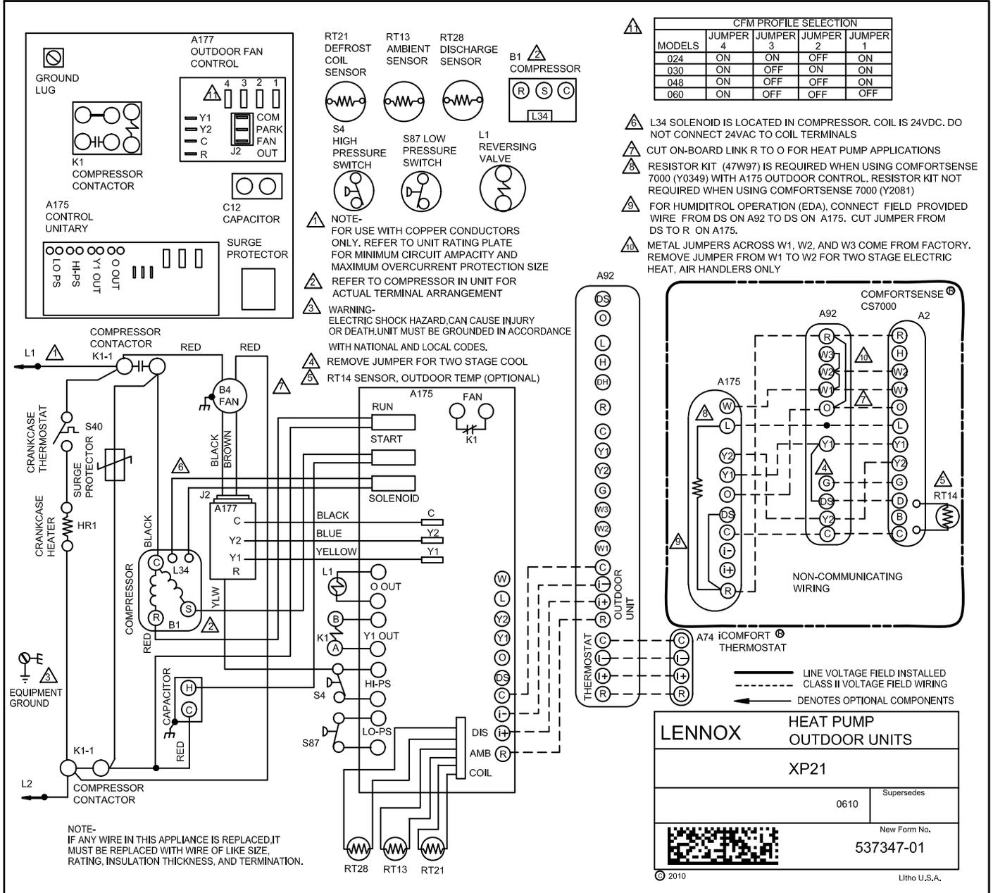
Figure 29. Typical XP21 Wiring (XP21-XXX-230-01 only)
