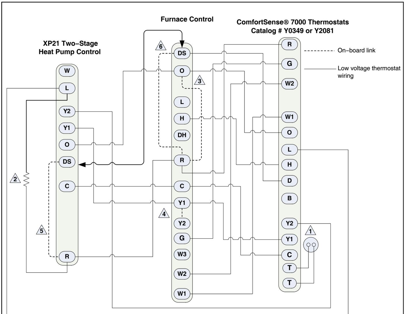
1. Thermostat **T** terminals are used for outdoor sensor input. Use for thermostat's outdoor temperature display (optional).
