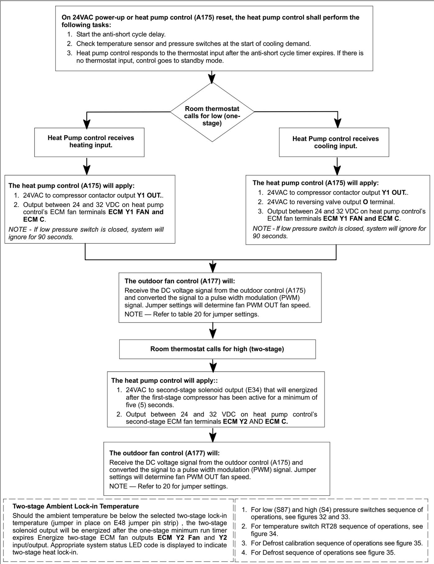
**Figure 31. One- and Two-Stage Cooling Sequence of Operations**
