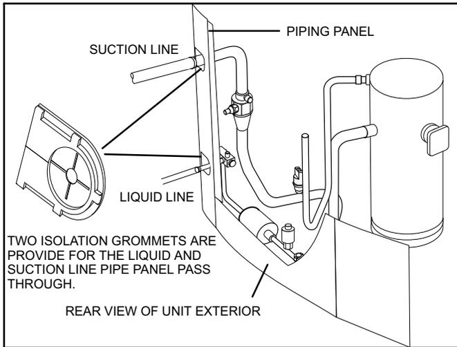
Figure 10. Isolation Grommets
