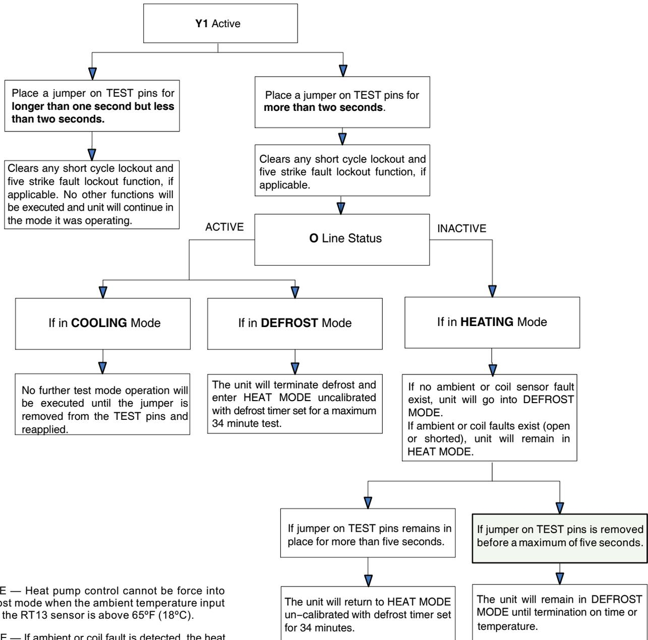
NOTE — Heat pump control cannot be force into defrost mode when the ambient temperature input from the RT13 sensor is above 65°F (18°C).
