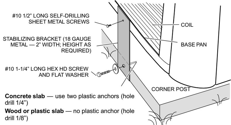
**Concrete slab** — use two plastic anchors (hole drill 1/4")
