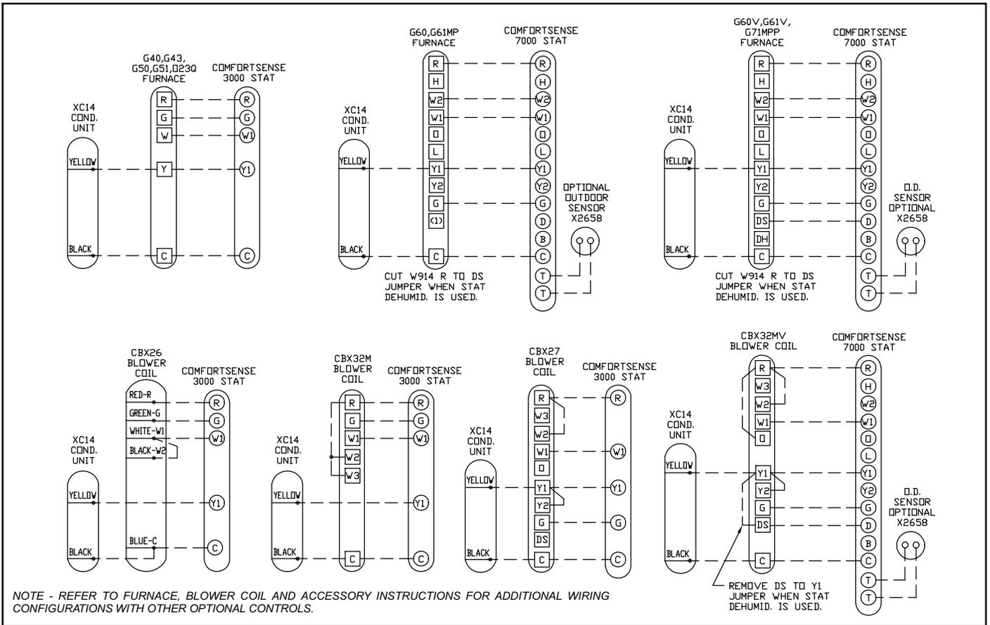
Figure 13. 24VAC Control Wiring Diagrams (Field Installed)
