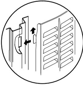
**IMPORTANT!** DO NOT ALLOW PANELS TO HANG ON UNIT BY TOP TAB. TAB IS FOR ALIGNMENT AND NOT DESIGNED TO SUPPORT WEIGHT OF PANEL.
