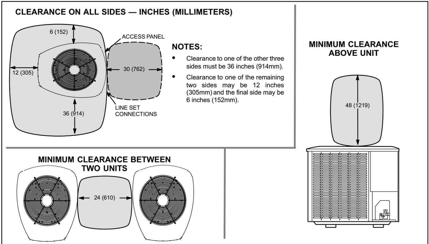
**Figure 3. Installation Clearances**
