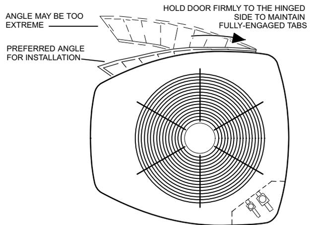
Figure 5. Removing and Installing Panels
