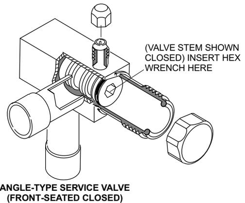
WHEN SERVICE VALVE IS **CLOSED**, THE SERVICE PORT IS OPEN TO THE LINE SET AND INDOOR UNIT.
