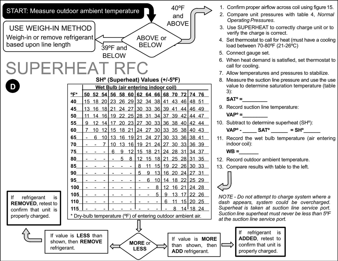
**Figure 20. Using HFC-410A Superheat (Fixed Orifice) Charge Method**
